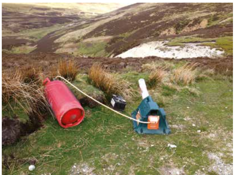
Propane gas gun bird scarers on Hopetoun Estate (Leadhills) Photo: Raptor Persecution Scotland
